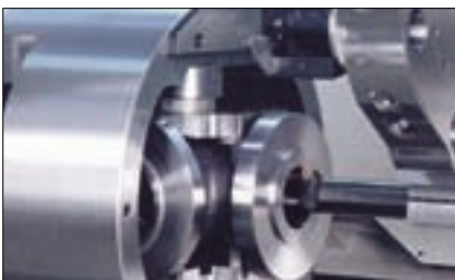
Hydraulically operated indexing chuck HSFK with correction piston
