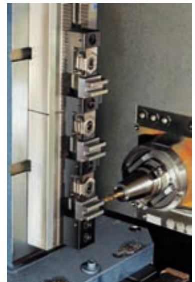
Locating- and intermediate jaws (width 45 mm) are specially designed for 3-side machining of small, narrow workpieces.
